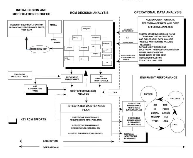
Figure 12-2: R&M/RCM Based Sustained Maintenance Planning Process
